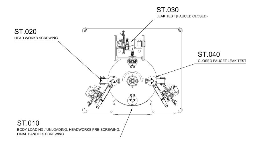
ASSEMBLY AND TEST MACHINE FOR TRADITIONAL FAUCET (HEADWORKS)
