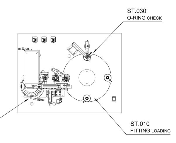
ST.020 O-RING LOADING AND GREASING
