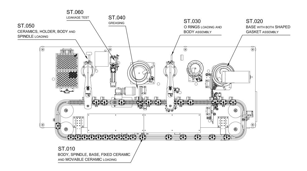
ASSEMBLY AND TEST MACHINE FOR CERAMIC CARTRIDGES
