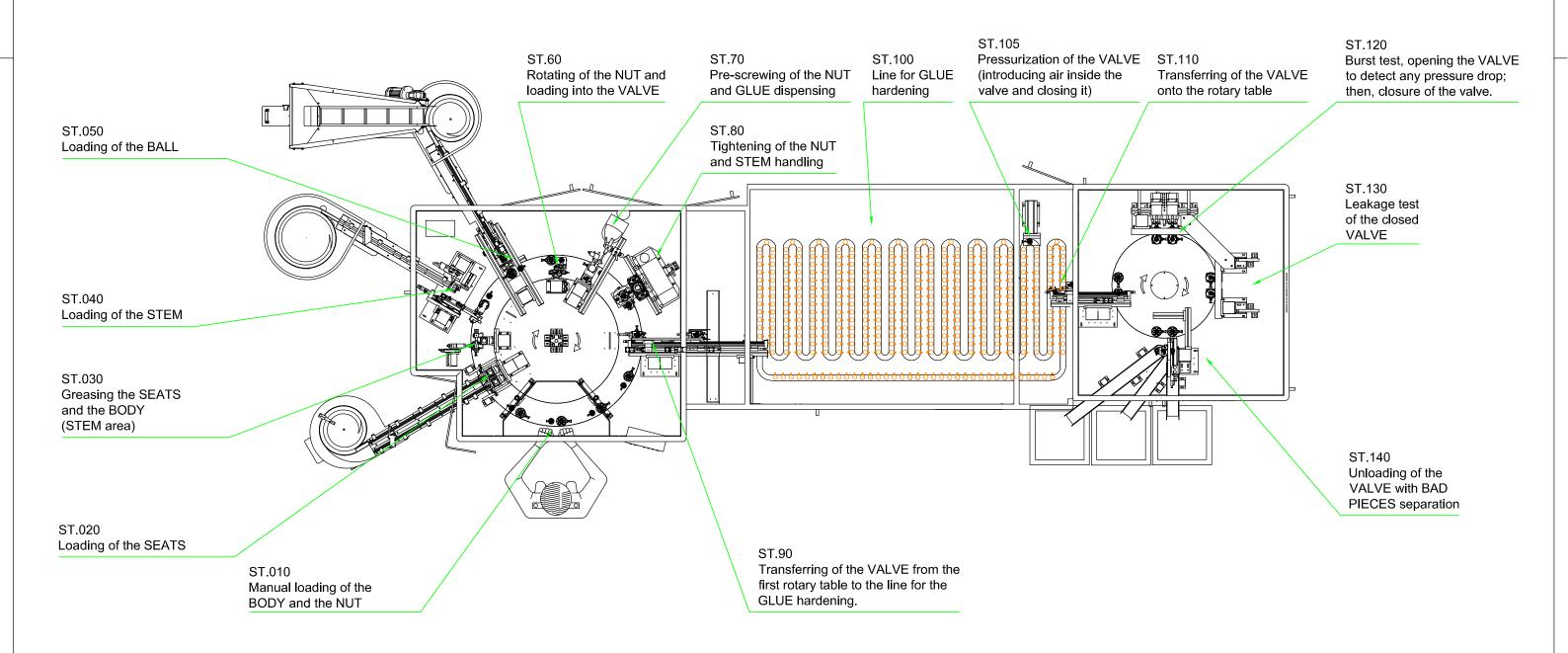
ASSEMBLING and TESTING MACHINE for 1/2" and 3/4" BALL VALVES
