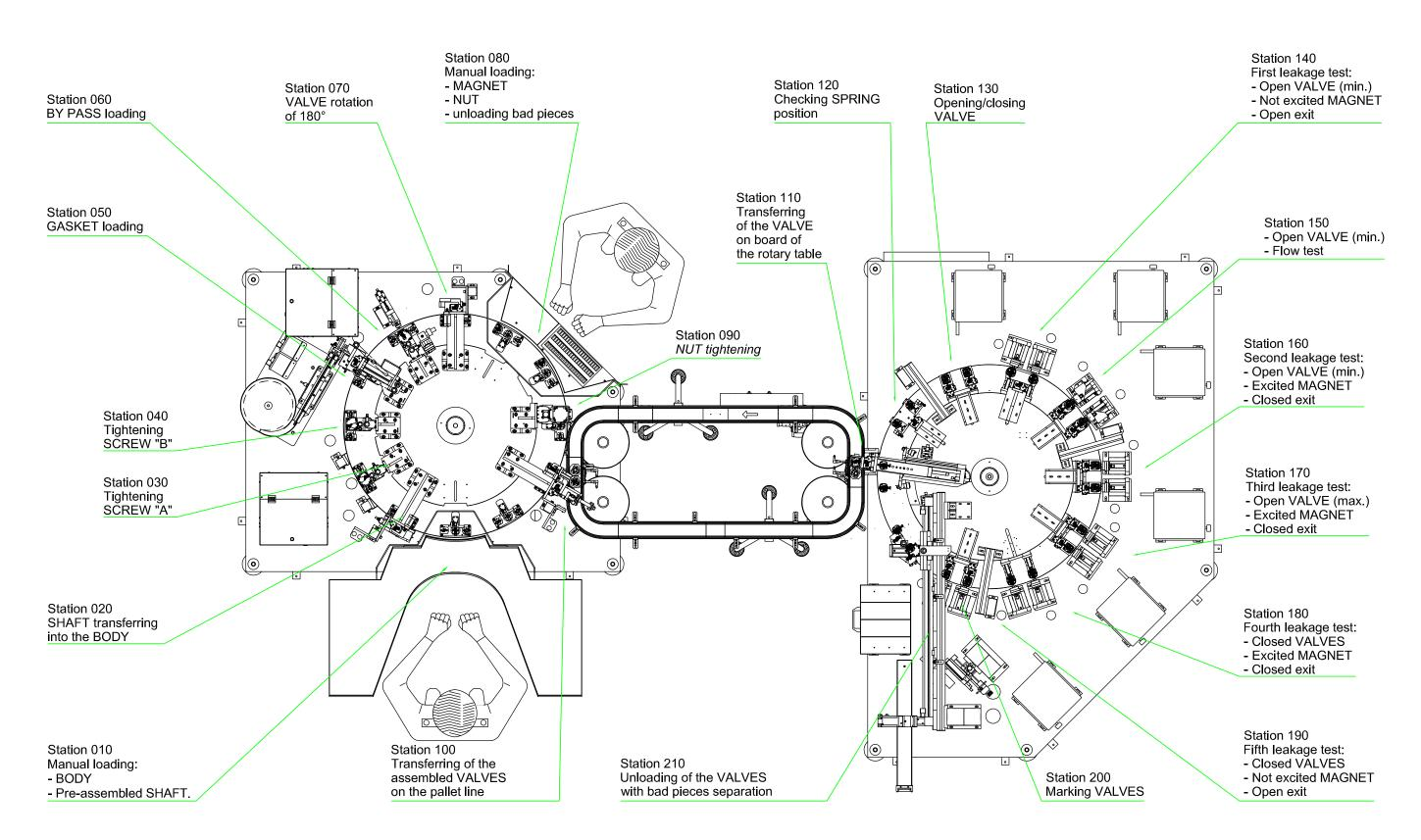
ASSEMBLY, CALIBRATION and TESTING MACHINE for GAS TAPS
