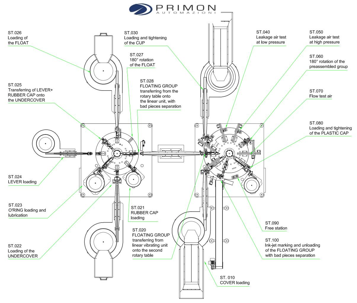
ASSEMBLY & TESTING "AIR VENT" RELIEF VALVES
