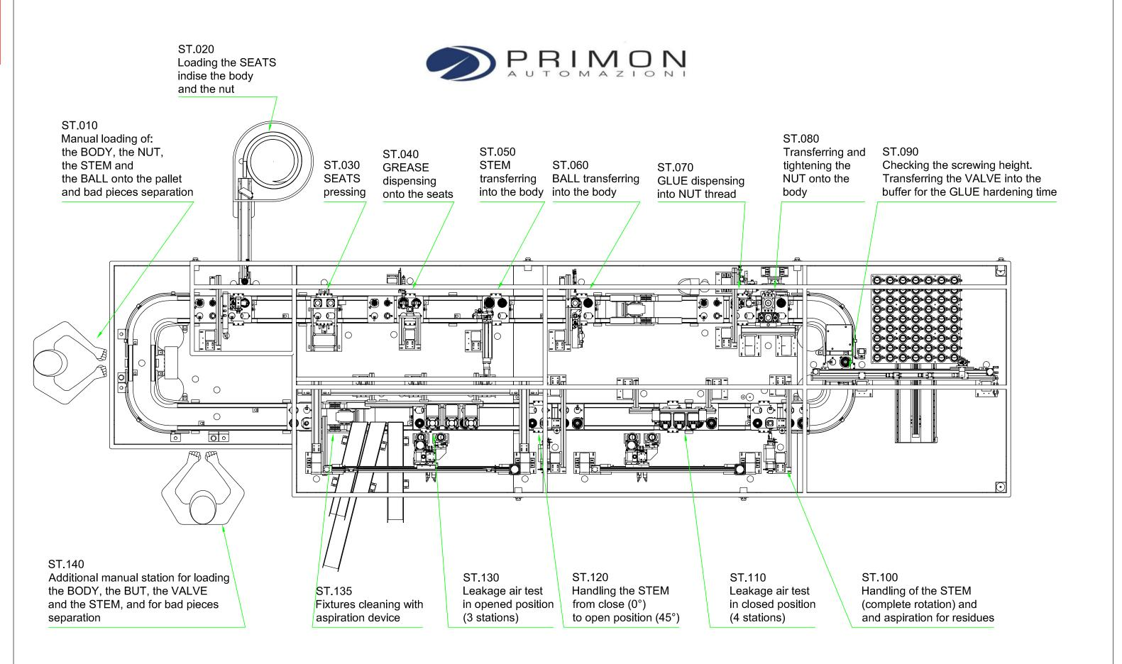
BALL VALVES (1/2" - 3/4" - 1") ASSEMBLING and TESTING MACHINE
