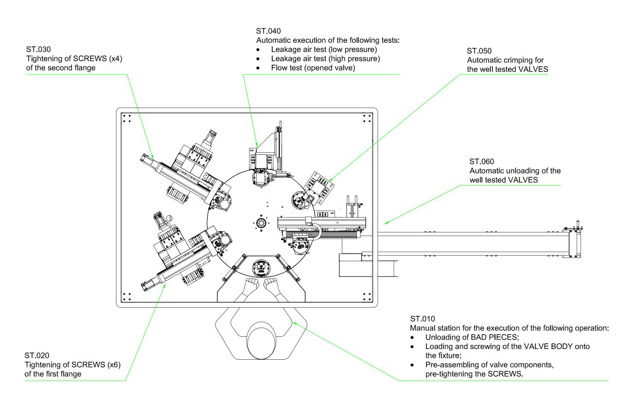
6" and 8" DIAPHRAGM VALVE ASSEMBLING and TESTING MACHINE
