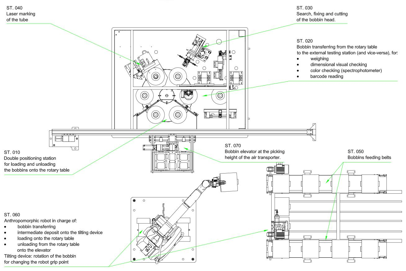
ROBOTIC CELL FOR BOBBINS MANIPULATION AND ROTARY TABLE FOR BOBBINS CONTROL
